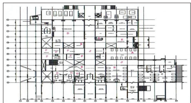
Figure 1: Ground floor plan of emergency block of study institute in north India. A: Hall A Emergency Medical Out Patient Department (EMOPD); B: Hall B EMOPD; C: Emergency Surgical Out Patient Department; D: Waiting hall; E: Chemist shop; F: Laboratory; G: Ultrasonography room; H: X-ray room; I: Reception; J: Corridors; K: Waiting area for patients
